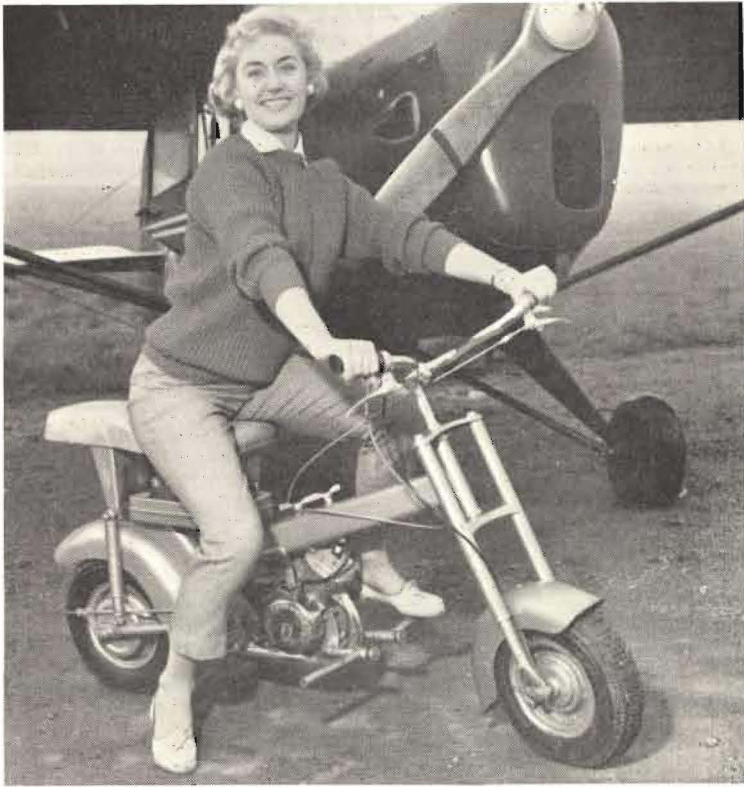
The assembled scooter weighs 65 lb. and does 180 miles per gallon.
