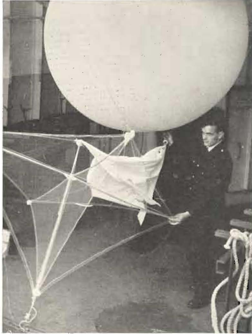
Preparing a meteorological balloon for ascent in the after hangar on Weather Explorer. The radio-sonde itself is attached below the kite-like radar reflecting screen.
